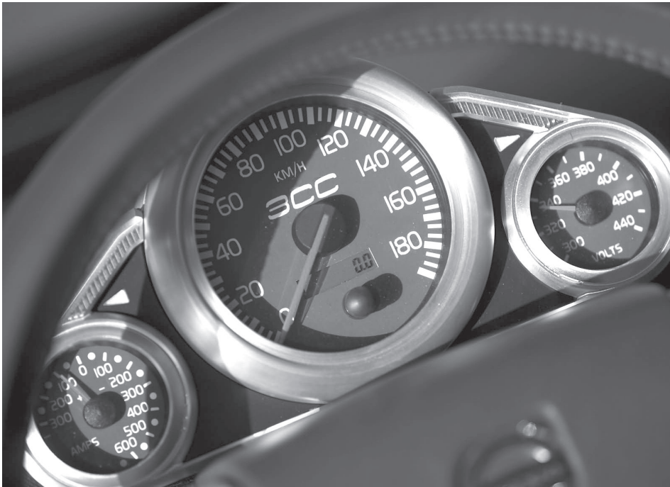
EV dashboard with +/- Amps on left, pack Volts on right.
