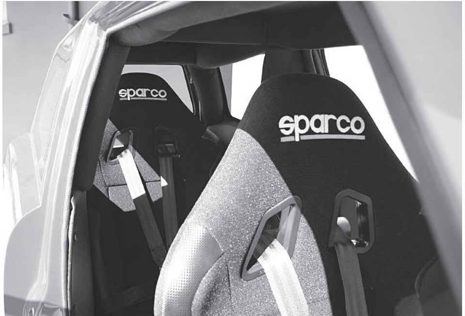
Tandem seating with 4-point seatbelts.
