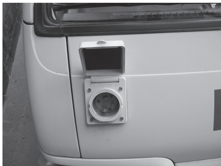
Charging port inlet, open
