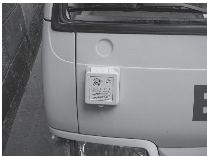
Charging port inlet, closed.
