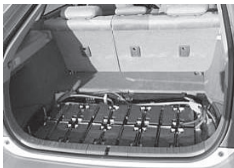
Battery pack expansion for plug in ability.
