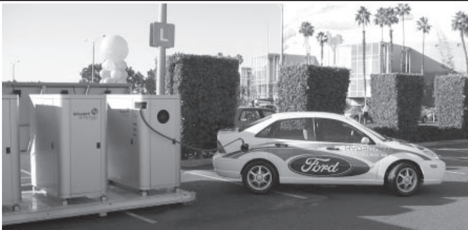
Stuart Energy Electrolized hydrogen refueling station, Ford refuels one of their fcv prototypes. The two hose cable for refueling, one for the refule, the smaller for sensing the tank pressure.
