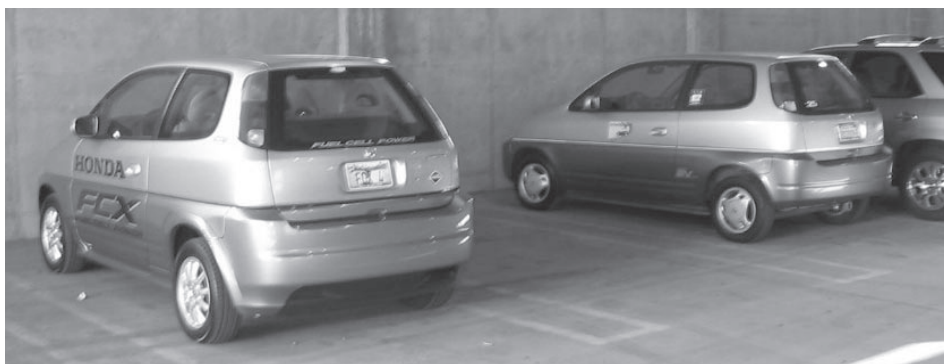
A side by side comparison of the canceled battery Honda EV plus and the Honda FCX fcv prototype. Note FCX uses EV plus chassis.
