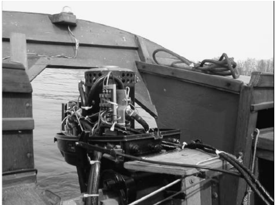
Electric ADC motor mounted to the existing outboard housing
