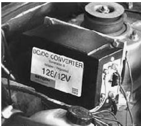
DC/DC Converter, draws 12v off pack.
