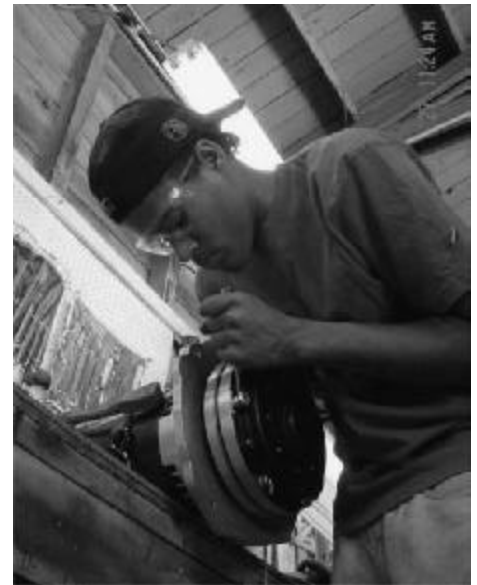
Solomon installing adaptor and flywheel
