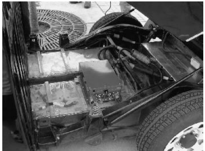
Under the tilt-bed are the YT batteries and a new PFC-20 charger.
