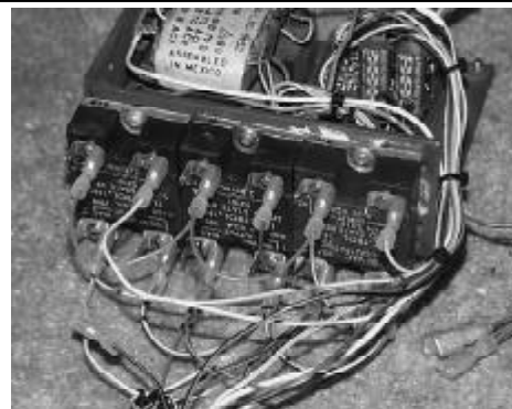
Assembled controller, consisting of solid state relays and the power connections
