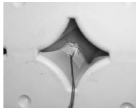
Fig 2: Temperature sensor taped to battery
