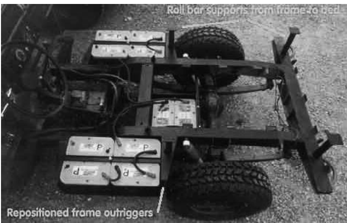
View of rear frame for battery layout.
