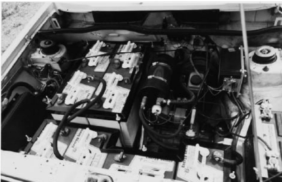
Battery rack layout in VW Rabbit - conversion kit by Electro Automotive
