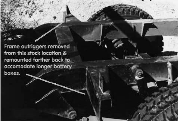
Frame modifications to accommodate batteries.
