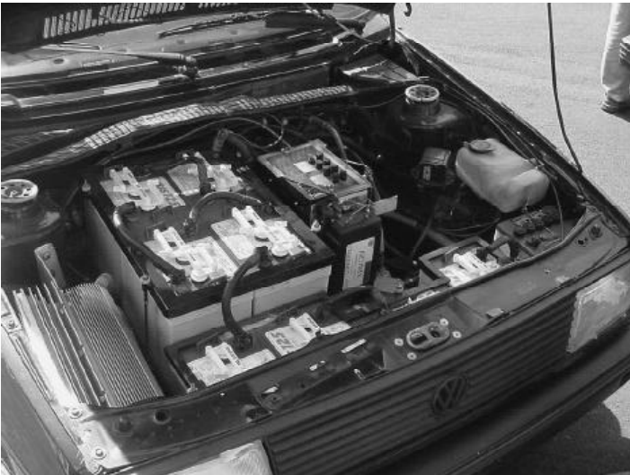
Excellent layout of engine (below), controller (left), batteries and more. VW's provide great fit for all the components.
