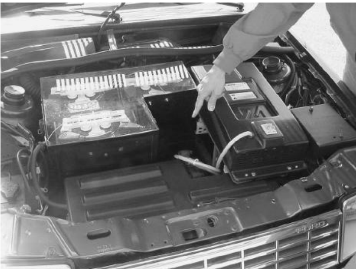
Clean front layout, with plastic display covers over batteries.
