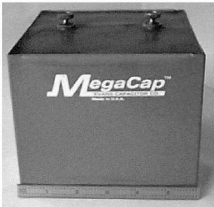
This hefty ultracapacitor has a rating of 65F, 14V.
